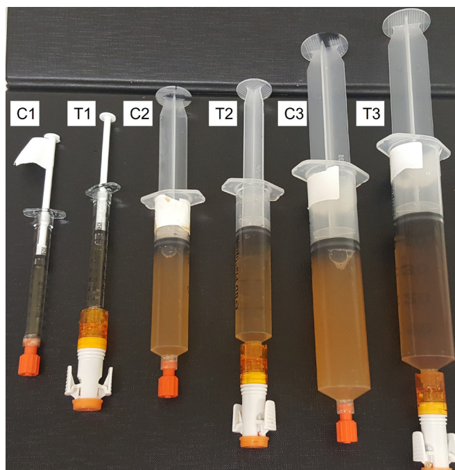
Figure 2 One of each size of Luer-Lock syringe fitted to either a blind hub as a positive control (C1, C2, C3) or to a Chemfort SAL as test article (T1, T2, T3) combinations post 14-day incubation at 30–35°C. SAL, syringe adaptor lock.
